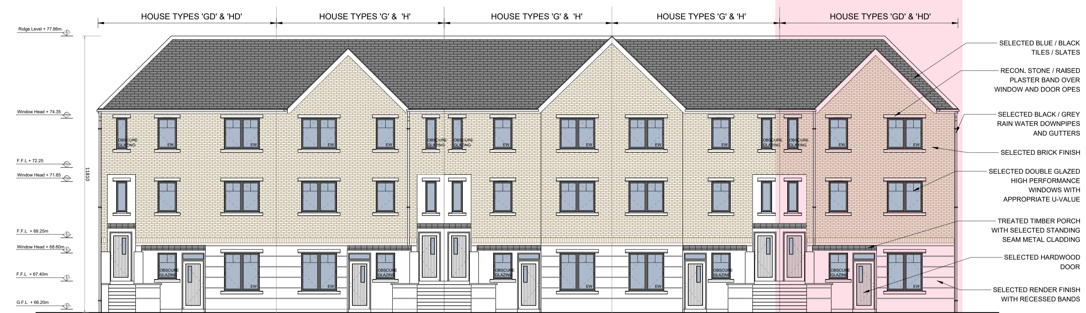
SOUTH EAST ELEVATION - BLOCK B
